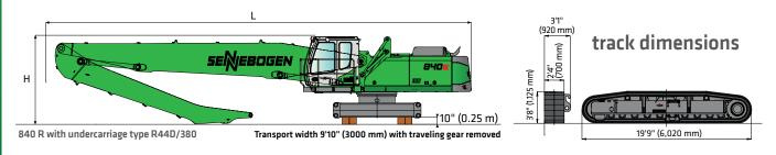
transport dimensions valid for boom position 1 only • boom position 2 may increase transport height & transport length • handrails, catwalks & other accessories are disassembled for transportation • \*optional cab E300/260 will increase machine transport height by 2" (50 mm)
