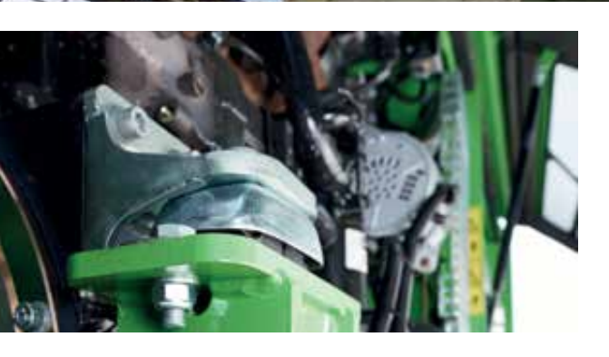
Low-vibration engine mounting reduces wear on components and lowers sound levels.
