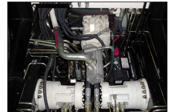
The cab tilts back to reveal quality components in an efficient layout. Steel lines improve serviceability and help dissipate heat.
