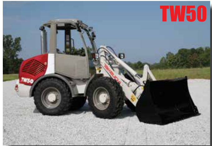
The TW50 weighs 8,708 lbs, and has 57 hp (gross)
