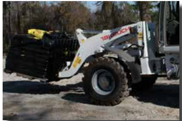
Center frame oscillation allows the loader to oscillate a total of 20° and helps to maintain stability and traction
