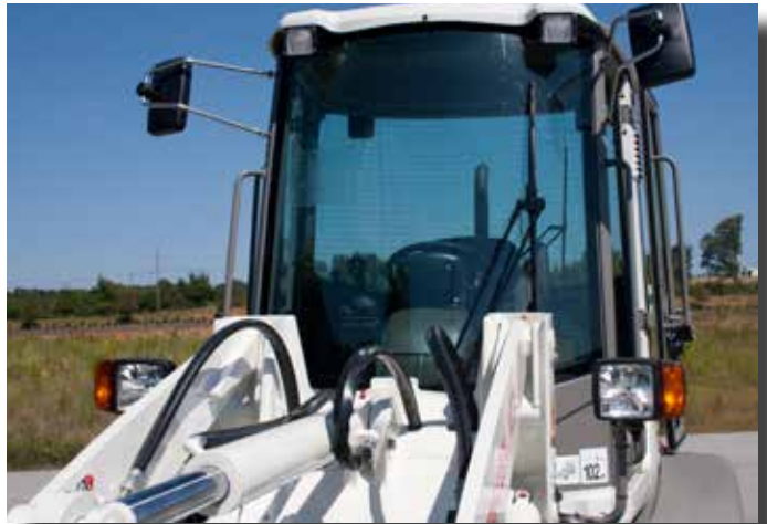
Protected hose routing and steel lines help reduce the chance for damage during operation
