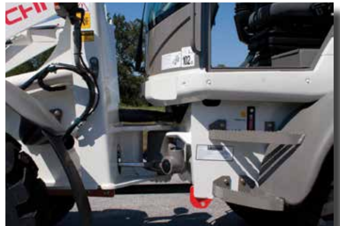
True center pivot steering provides a total angle of 80 degrees and allows rear wheels to follow in same track as front wheels enabling the machine to maneuver in tight areas
