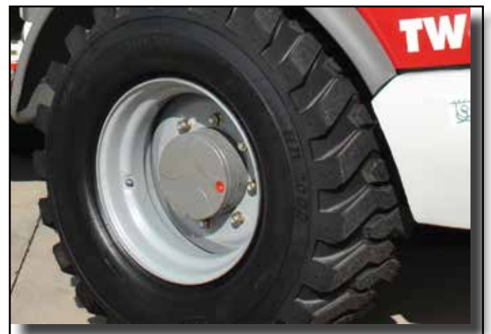
Outboard planetary final drives allow for easy servicing and help keep the oil and components cool and clean
