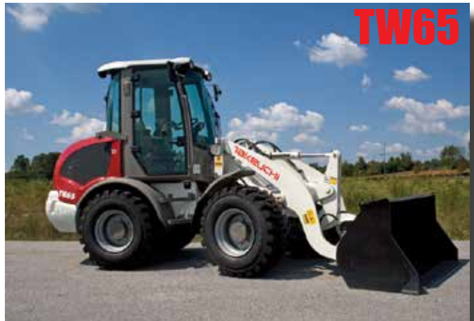
The TW65 weighs 10,582 lbs, and has 69 hp (gross)
