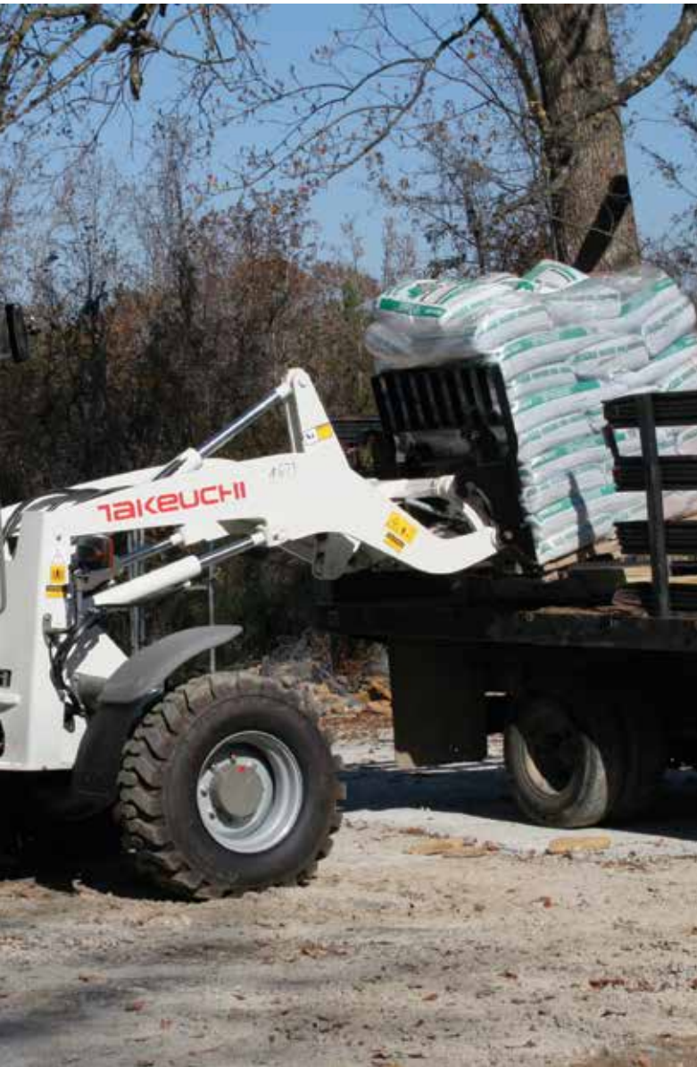
True center pivot steering provides a total angle of 80 degrees and allows rear wheels to follow in same track as front wheels enabling the machine to maneuver in tight areas
