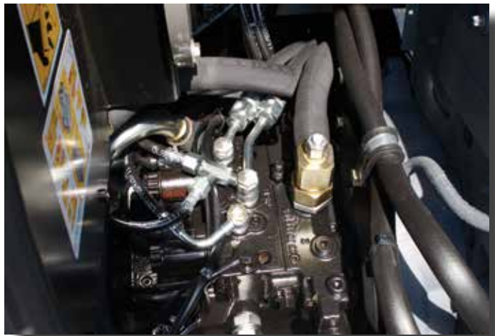
Convenient hydraulic system test ports provide an easy connection for diagnostic equipment to ensure your machine is running at its peak performance
