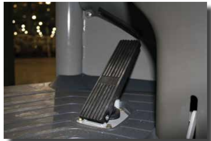
Travel speed is easily controlled using the 100% inching pedal that can slow the loader to a crawl/stop, reducing wear on the brakes and improving fuel economy
