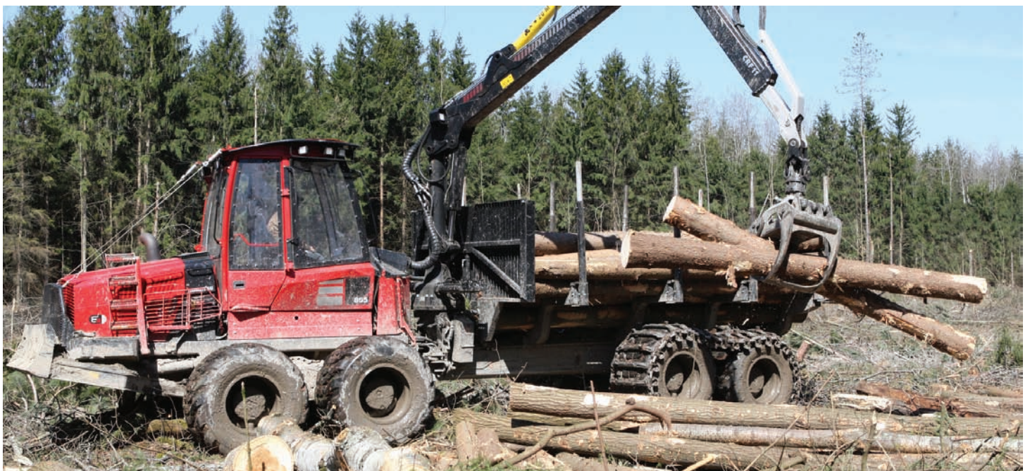
The Komatsu 865 8-wheel forwarder carries 16.5 tons. The advanced HST transmission optimizes traction and maneuverability.
