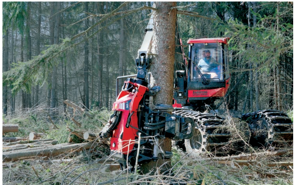
Owner/operator, Brock Stadler says the 365.1 head on the 2015 Komatsu 911.5 harvester is fast and accurate. He appreciates its simplicity, durability and power.
