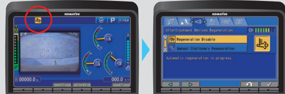
Aftertreatment device regeneration screen
