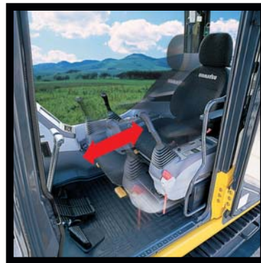
Seat Sliding Amount: 340 mm 13.4", increased 120 mm 4.7"
